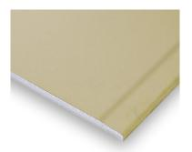
**Product description:** Gypsum plasterboard acc. to DIN EN 520, type DFH2IR, moistureresistant, made of a gypsum core with high surface hardness, dense gypsum core encased in cardboard.
